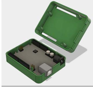
Fig. 2. 3D model of enclosure for Arduino Uno board.
